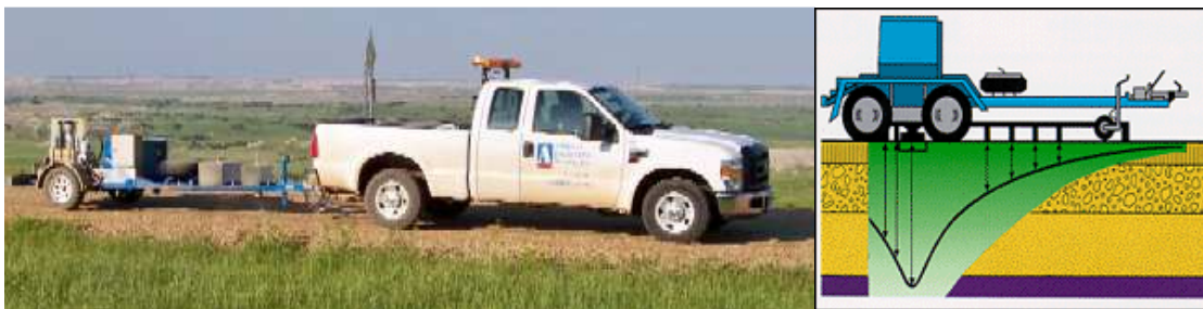
Figure C1 Dynatest 8002 FWD Test System
