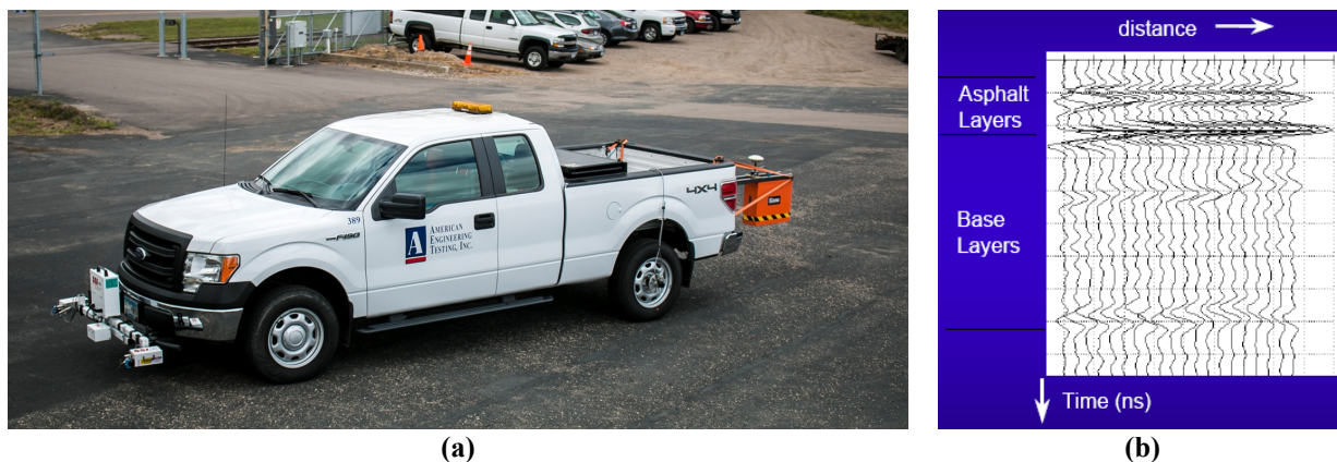
Figure B1. (a) GSSI 2 GHz Air-coupled GPR Test System mounted to the rear of an AET survey vehicle and (b) example of raw data collected using the GPR test system
